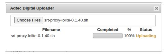
To execute the application for the first time, the user must SSH into the Adtec device and run the *srt-proxy-<host platform>-x.yy.zz.sh* file. Do NOT upload the .zip file to the Adtec.
