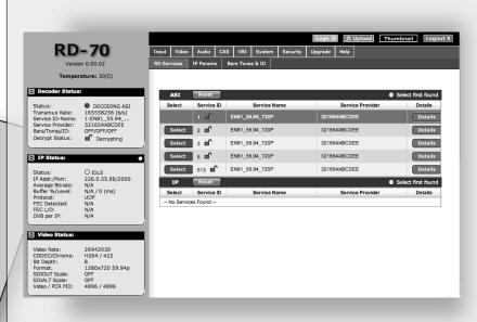
Note: IP service selection is treated differently than ASI or RF inputs. To populate the IP services section, you need to first visit the IP Params tab and set the correct Rx Address, port and handling parameters. Return to the RD Services tab. Click the 'Select First Found' radio button for IP. This will populate the RD Services tab with services found on the IP input.
